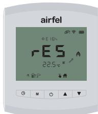
With the “▲ 4” and “▼ 5” buttons, you can switch between “①” info menu, “⚙️” parameters and “📅” weekly schedule and “⚠️” error history. You can go to the desired menu setting by pressing “○ 3”.
