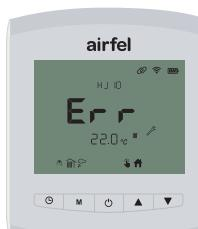
In this case, if the “▲ 4” up button is pressed, then “rES” text starts blinking on the screen. In the meantime, if the “▲ 4” button is pressed once more, the reset request is transmitted to the boiler. If the cause of the error has disappeared, the boiler returns to normal operation.
